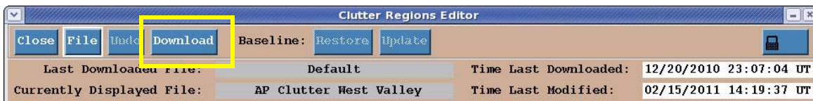
Figure 1-16. Once the correct Clutter Regions file has been selected, it can be downloaded to the RDA by clicking the Download button (yellow box).
