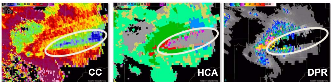
Figure 2-19. Low CC values (left) due to non-uniform beam filling can also impact the derived products like the Hydroclassification product (middle) and the Digital Precipitation Rate (right).
