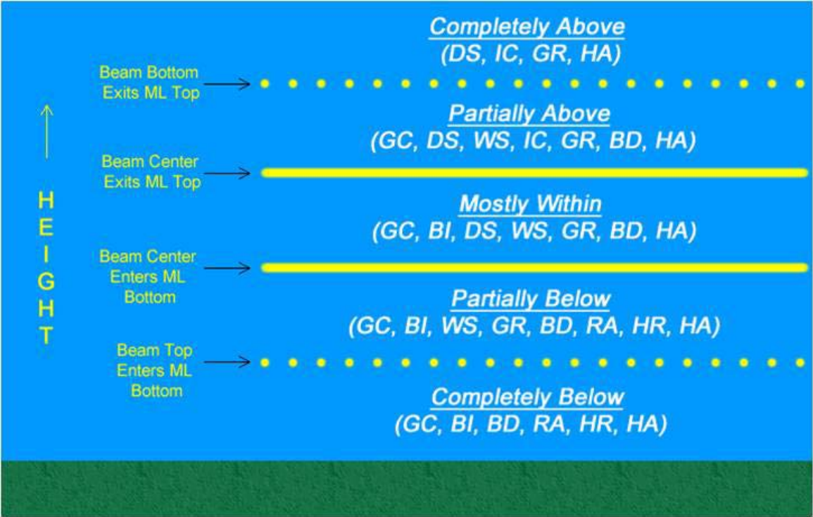
Figure 2-12. Graphic illustrating the method of using the melting layer to determine hydrometeor classification.
